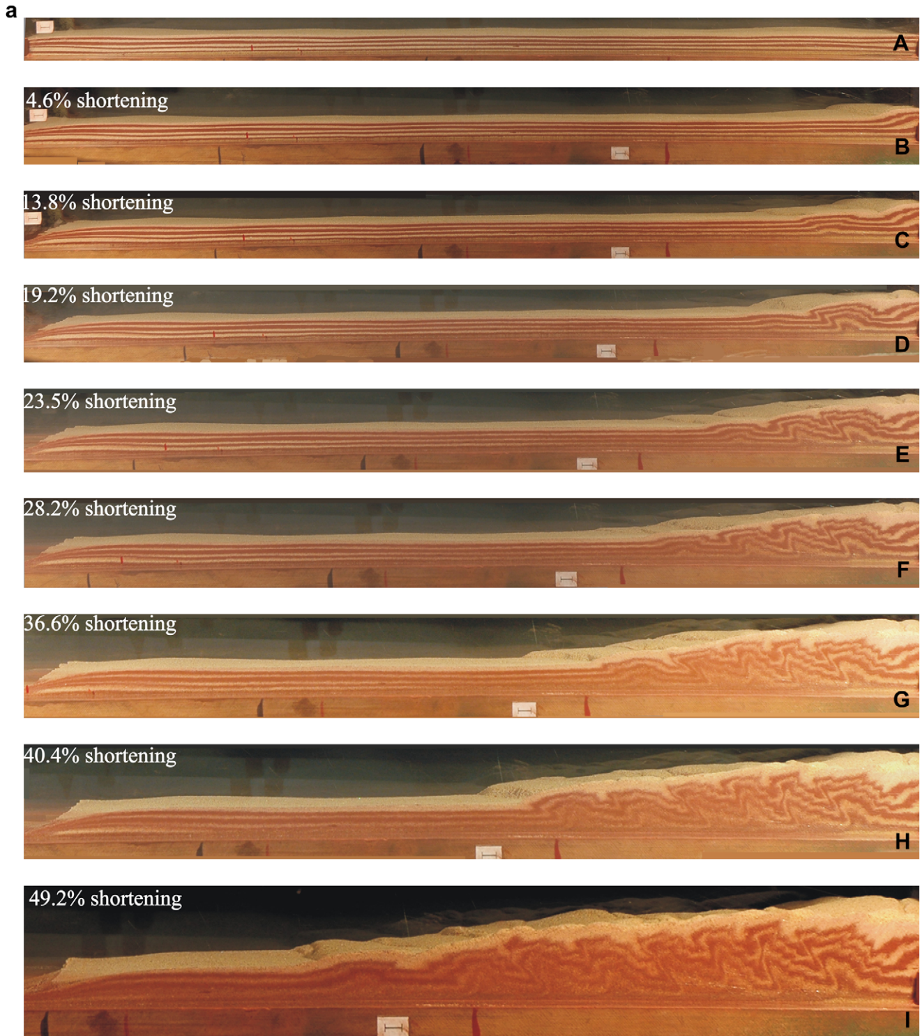
Fig. 3. Progressive development of imbricate thrust systems in sand models with (a) low ( \mu_b = 0.36 ), (b) moderate ( \mu_b = 0.41 ) and (c) high ( \mu_b = 0.46 ) basal friction. Note that frontal thrusts in (c) show a strong variation in their spacing. Models were deformed by horizontal contraction (right to left). Scale bar: 1 cm.
